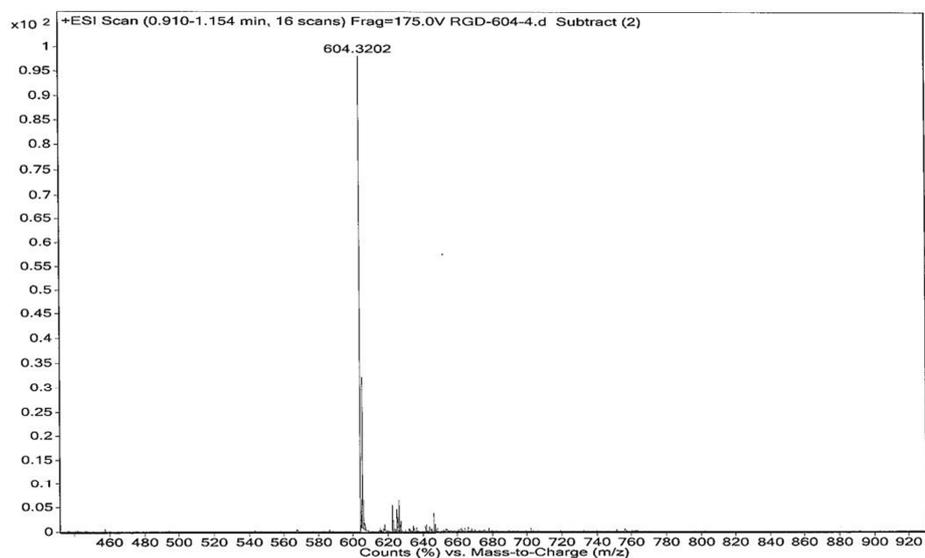
**Fig. S7. Mass spectrometry analysis** of of cRGD (HRMS-ESI: m/z  $C_{27}H_{41}N_9O_7$   $[M+H]^+$  604.3202, found 604.3202.)
