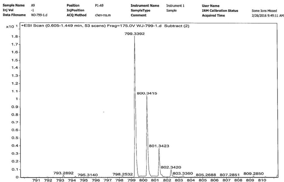
**Fig. S11.** Mass spectrometry analysis of SiPc-PQ 2 (HRMS-ESI:  $m/z$  calcd for  $m/z$   $C_{44}H_{42}N_{12}O_2Si [M+H]^+$  799.3396, found 799.3392).
