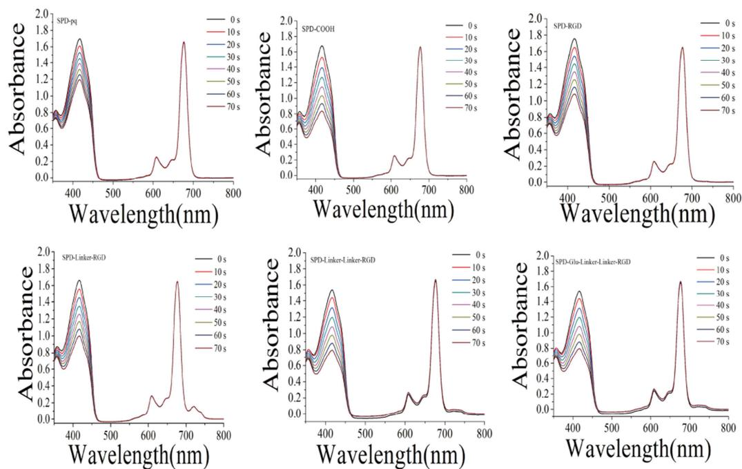
**Fig. S4.** Typical spectra for determination of the singlet oxygen quantum yield of SiPc-PQ **2**, SiPc-COOH **3**, RGD-SiPc **4**, RGD-Linker-SiPc **5**, RGD-(Linker)<sub>2</sub>-SiPc **6** and RGD-(Linker)<sub>2</sub>-Glu-SiPc **7** in DMSO using DPBF as a singlet oxygen quencher. DPBF concentration =  $2 \times 10^{-5}$  M.
