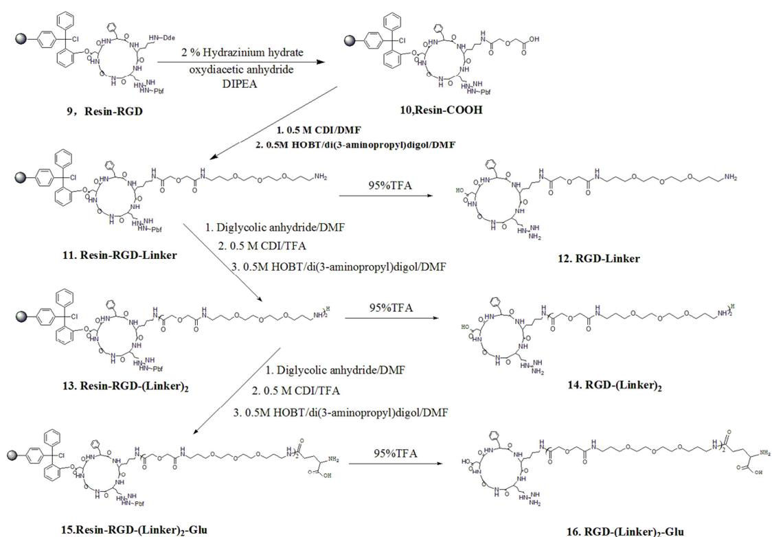
Scheme S2. Synthetic procedure of cRGD, cRGD-Linker, cRGD-(Linker)<sub>2</sub> and cRGD-(Linker)<sub>2</sub>-Glu
