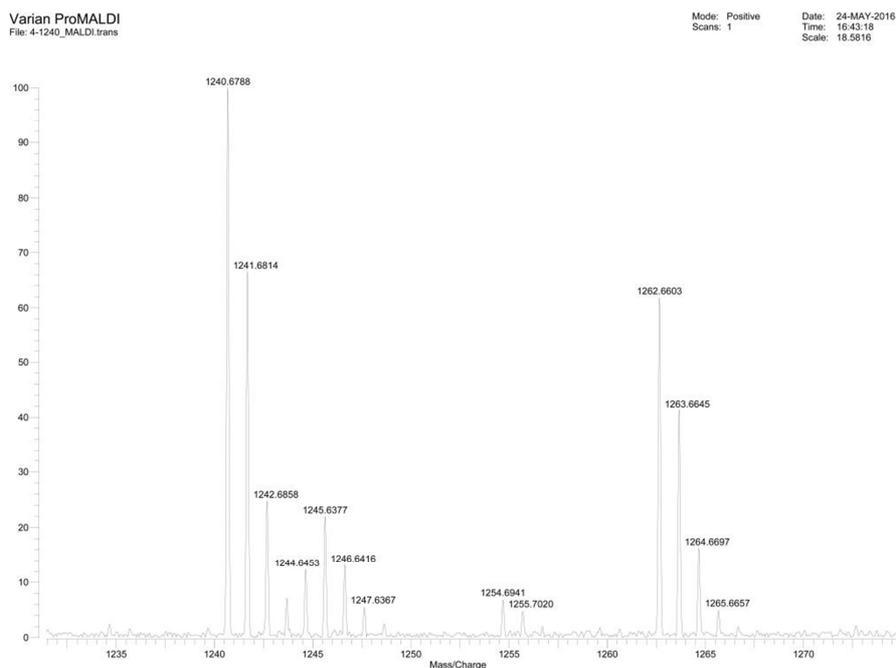
**Fig. S9.** Mass spectrometry analysis of RGD-(Linker)<sub>2</sub> (HRMS-ESI: m/z calcd for m/z C<sub>55</sub>H<sub>93</sub>N<sub>13</sub>O<sub>19</sub> [M+H]<sup>+</sup> 1240.6783, found 1240.6788, calcd for C<sub>55</sub>H<sub>93</sub>N<sub>13</sub>O<sub>19</sub>Zn<sup>+</sup> [M+Na]<sup>+</sup> 1262.6603, found: 1262.6603).
