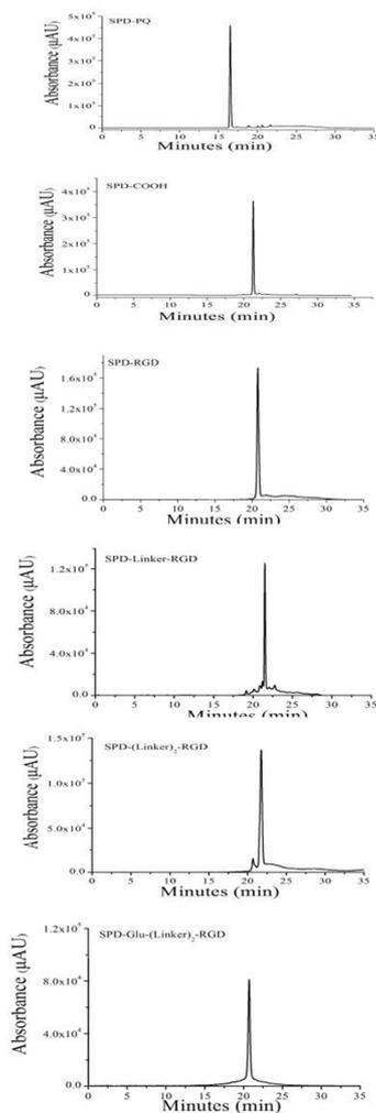
**Fig. S1.** HPLC analysis of SiPc-PQ **2**, SiPc-COOH **3**, RGD-SiPc **4**, RGD-Linker-SiPc **5**, RGD-(Linker)<sub>2</sub>-SiPc **6** and RGD-(Linker)<sub>2</sub>-Glu-SiPc **7**. Wavelength for detection: 668 nm. SiPc-PQ **2** ( $t_R = 16.5$  min), SiPc-COOH **3** ( $t_R = 21.3$  min), RGD-SiPc **4** ( $t_R = 20.8$  min), RGD-Linker-SiPc **5** ( $t_R = 21.5$  min), RGD-(Linker)<sub>2</sub>-SiPc **6** ( $t_R = 21.8$  min) and RGD-(Linker)<sub>2</sub>-Glu-SiPc **7** ( $t_R = 20.7$  min).
