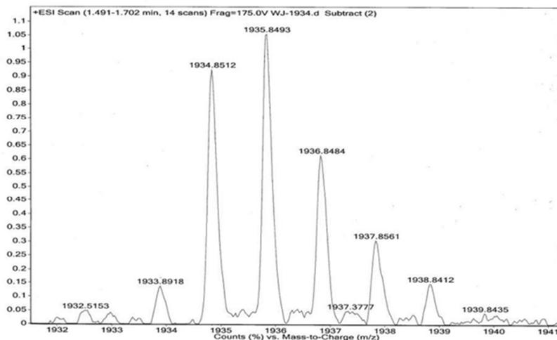
Fig. S14. Mass spectrometry analysis of RGD-Linker-SiPc 5 (HRMS (ESI): m/z calcd for  $C_{93}H_{116}N_{23}O_{22}Si [M + H]^+$  1934.8429, found 1934.8512).
