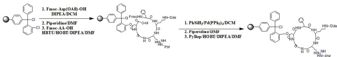
Scheme S1. Synthetic procedure of the resin-bonded cyclized cRGDfK peptide
