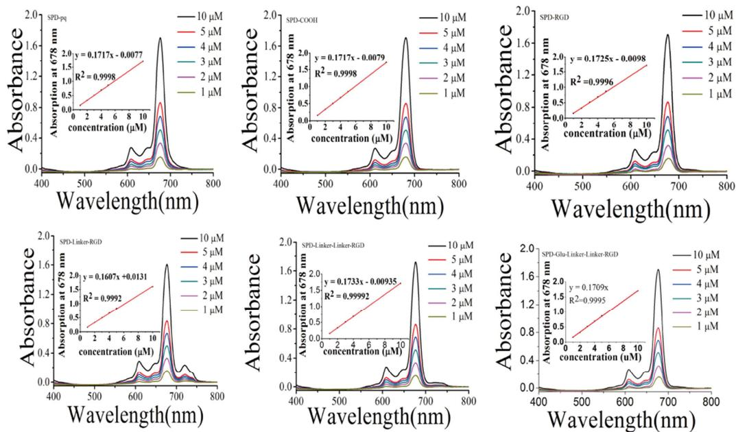
**Fig. S3.** Absorbance spectra of SiPc-PQ **2**, SiPc-COOH **3**, RGD-SiPc **4**, RGD-Linker-SiPc **5**, RGD-(Linker)<sub>2</sub>-SiPc **6** and RGD-(Linker)<sub>2</sub>-Glu-SiPc **7** at various concentrations in DMSO. The insets show plots of the intensity at 678 nm versus the concentration of the corresponding compounds.
