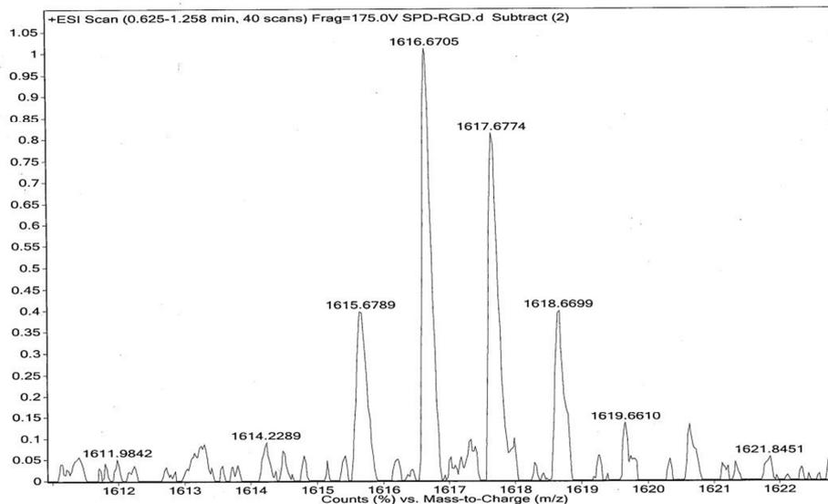
Fig. S13. Mass spectrometry analysis of RGD-SiPc 4 (HRMS-ESI: m/z calcd for m/z  $C_{79}H_{89}N_{21}O_{16}Si [M+H]^+$  1616.6638, found 1616.6705).
