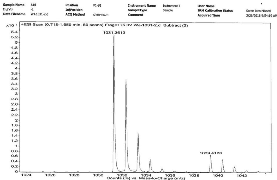
**Fig. S12.** Mass spectrometry analysis of SiPc-COOH 3 (HRMS-ESI:  $m/z$  calcd for  $m/z$   $C_{52}H_{50}N_{12}O_{10}Si [M+H]^+$  1031.3615, found 1031.3613).
