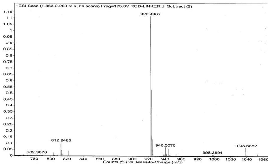
**Fig. S8. Mass spectrometry analysis** of cRGD-Linker (HRMS-ESI: m/z calcd for m/z  $C_{41}H_{67}N_{11}O_{13}$   $[M + H]^+$  922.4993, found 922.4987).
